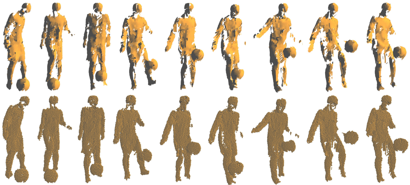
Fig. 9: Different poses of the “soccer (juggle)” 4D point cloud dataset rendered through surfels (top row) and voxels (bottom row).
