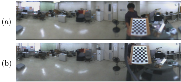
Figure 2. Panoramic image pair converted from omnidirectional image shown in the Fig. 1. (a): Upper image, (b): Lower image.
